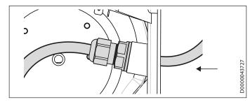
► Route the power cable through the cable gland from the back of the appliance.
