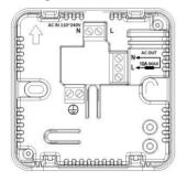
Connect the live and neutral AC mains (marked AC IN 110-240v). This feed should come from the fused spur.
